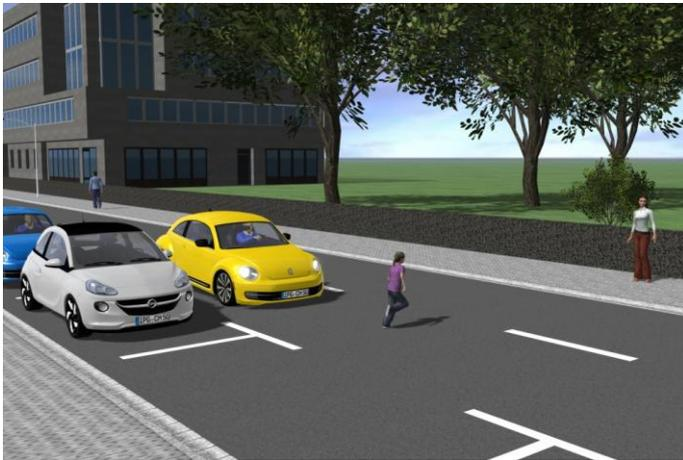
**Figure 1:** Euro NCAP-compliant test scenario for emergency brake assistant in CarMaker 5.0
